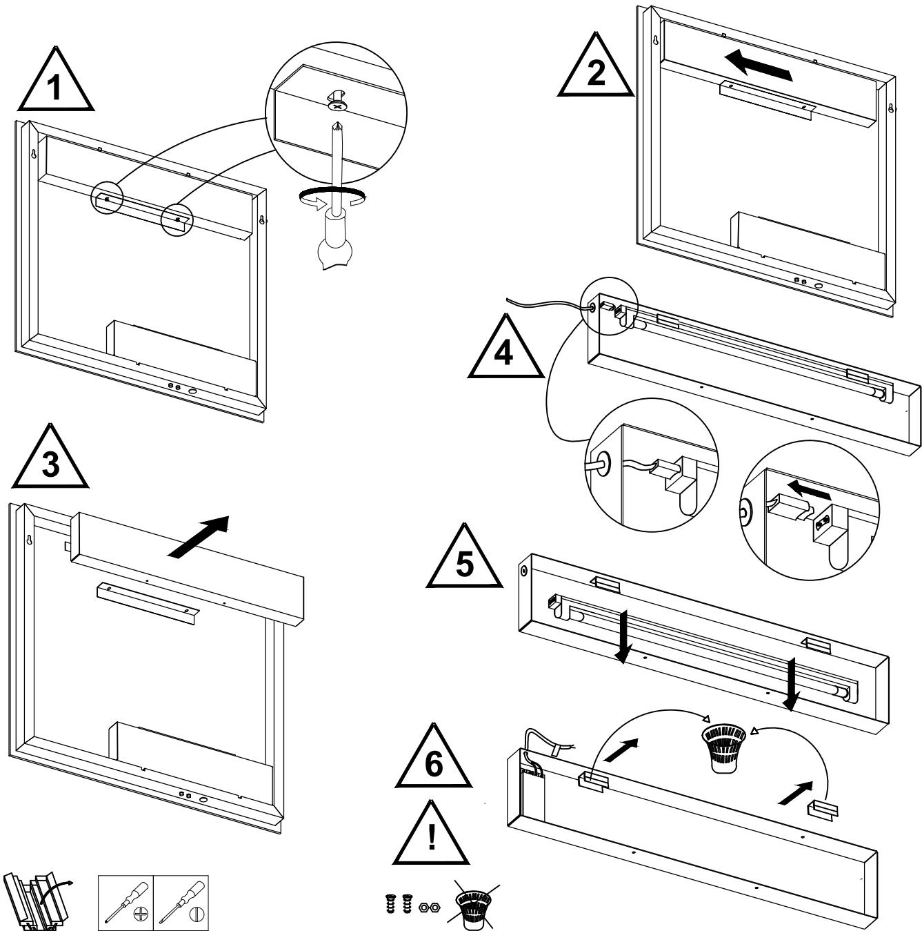
INSTALLER TUBE T5 13 W - HOW TO REPLACE BY NEW T5 13 W LIGTH TUBE:
